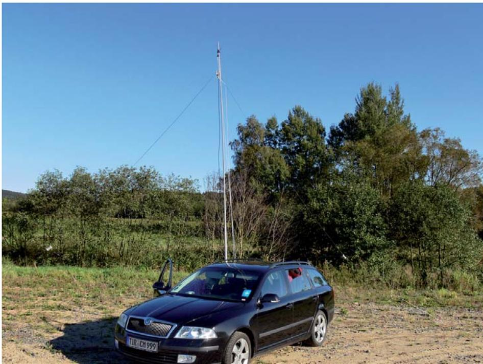
pulling upwards with the trap-dipole on the role
